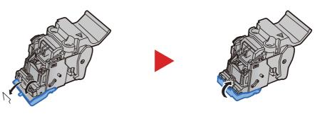
**5** Install the Staple Cartridge Holder (B) or (C).
