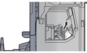
**3** Remove the Staple Cartridge Holder (B) or (C).
