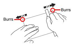
Before loading Hagaki (Cardstock), fan them and align the edges. Hagaki (Cardstock) should be fed from the MP tray with the print-side down or the cassette and the optional paper feeder with the print-side up. If the Hagaki (Cardstock) paper is curled, straighten it before loading. Printing onto curled Hagaki (Cardstock) may cause jams.
