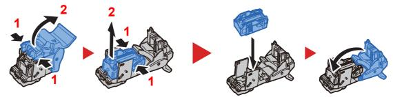
**1** Install the Staple Cartridge Holder (B) or (C).
