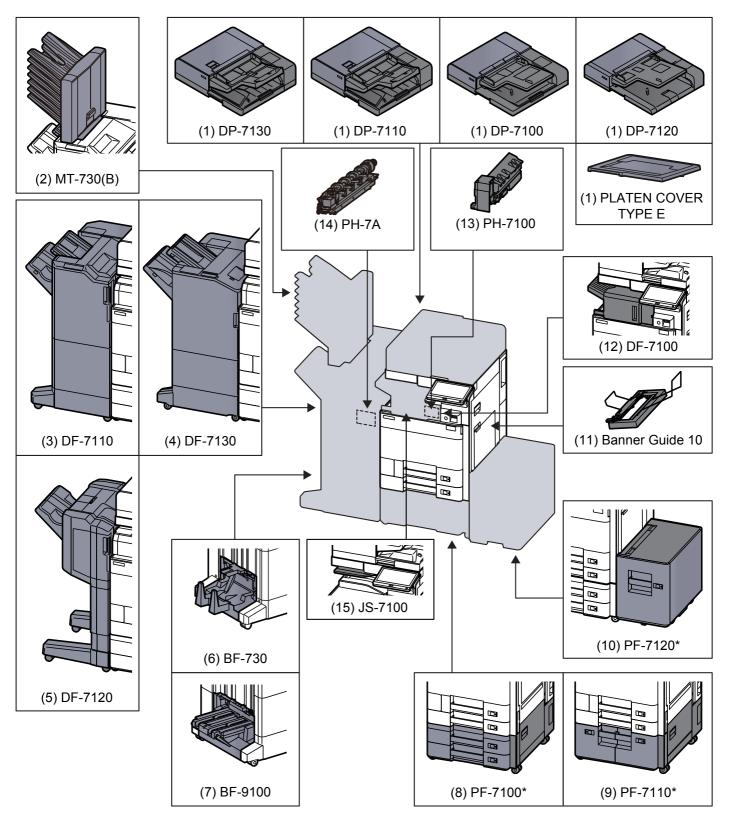
\* If the following option is installed, toppling prevention kit must be installed: PF-7100, PF-7110, PF-7120
