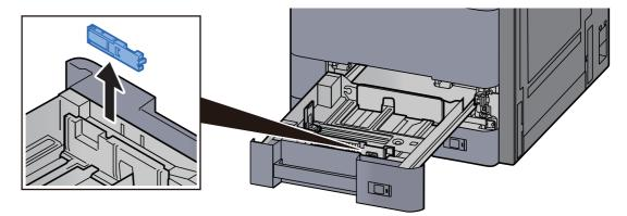
**3** Expand the lever of the envelope feed guide when loading envelopes larger than Envelope C5 which has a width of 162 mm (6.4").
