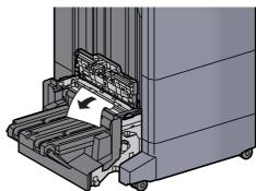
**11** Open the folding unit conveyor guide.
